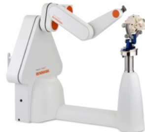
Stereotactic Robot for guiding cell transplantation into human brain
